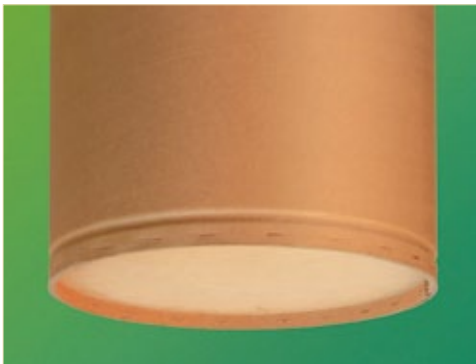
Tacked MDF bottom clamped and tacked between crimp and cardboard stop ring
